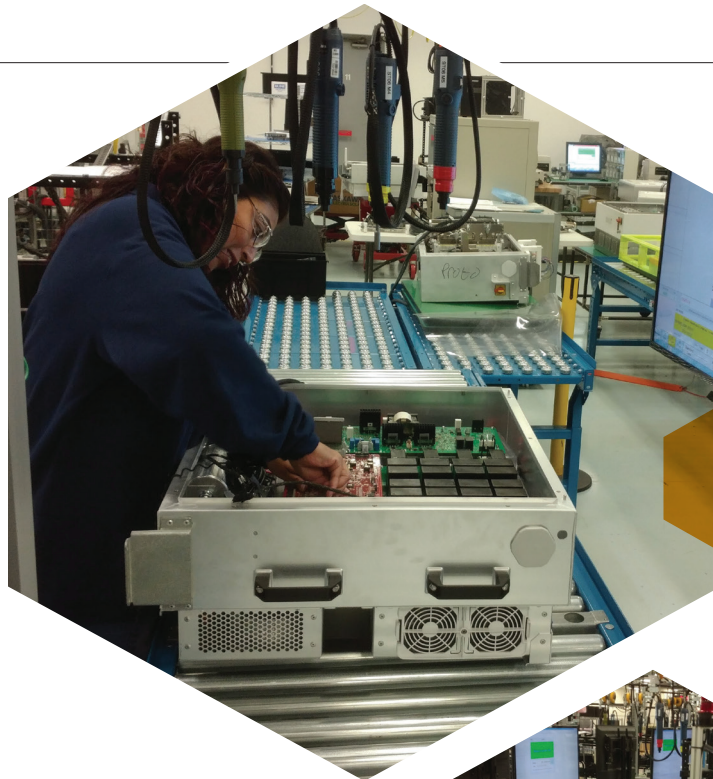
String inverters are assembled at Yaskawa America facilities in Buffalo. Solectria
