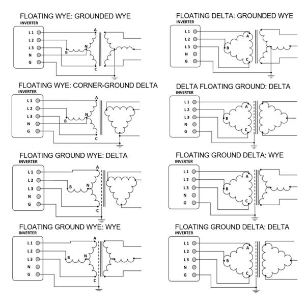
Figure 1. Permitted Transformer Configurations for XGI 1500-DCG Interconnection
