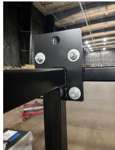
Fig. 3. Image and photo of the lifting eyes on the vertical elements of the POWERACK
