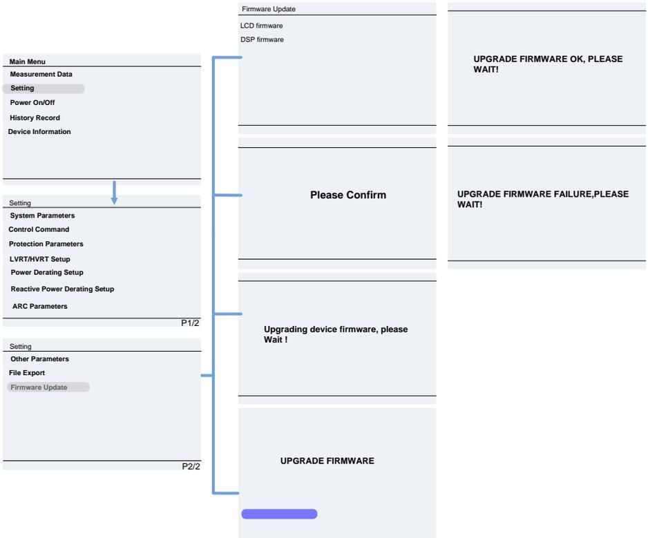
Figure 6.7 – Firmware Upgrade Interface
