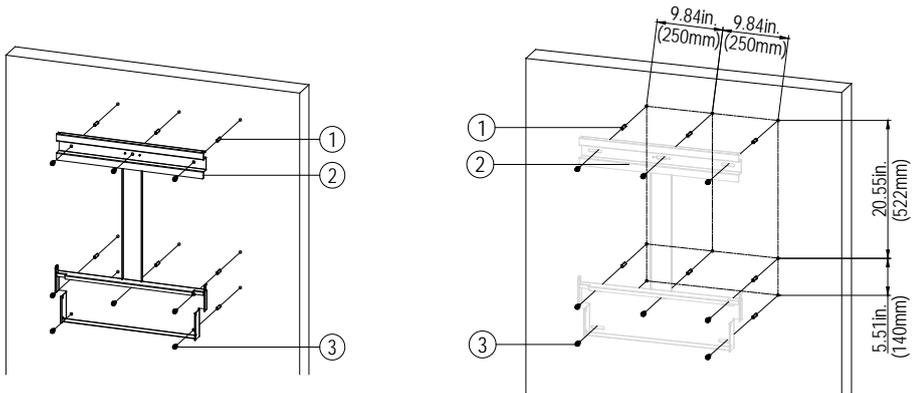
Figure 2.7 - Securing Mounting Bracket
