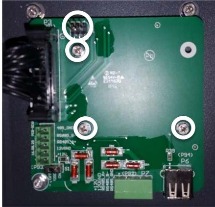
**Figure 2.47 - Communication Card and Location for Ethernet Network Card**
