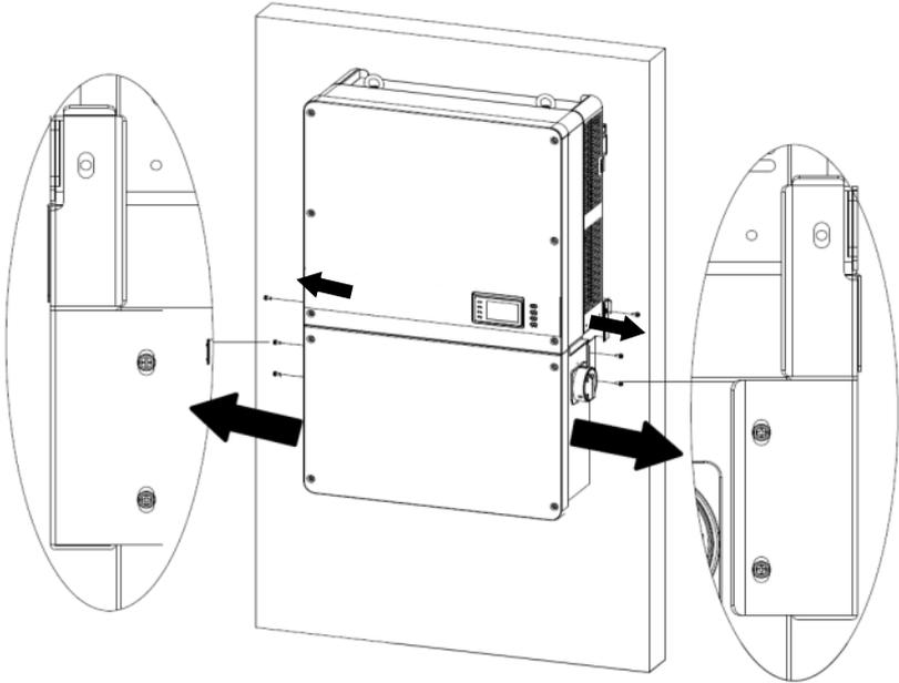
**Figure 6.3 - Remove the Screws on Both Sides**
