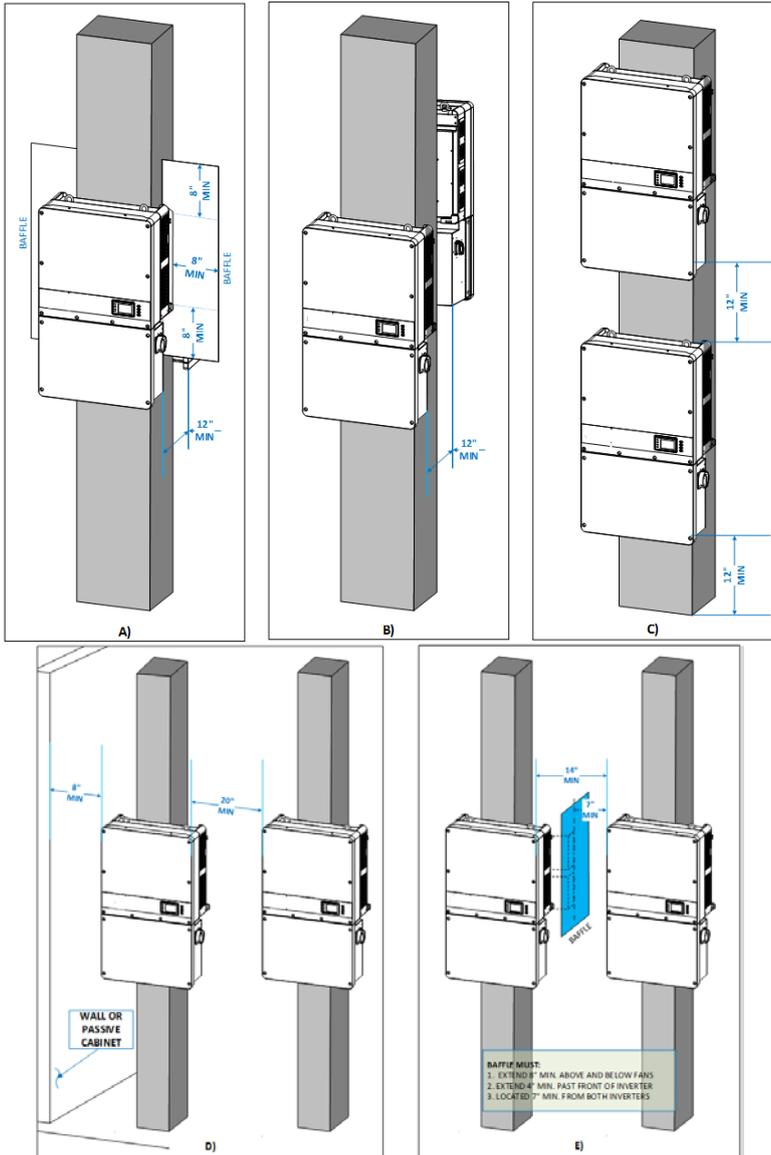
Figure 2.4 - Inverter Pillar Mounting Specifications
