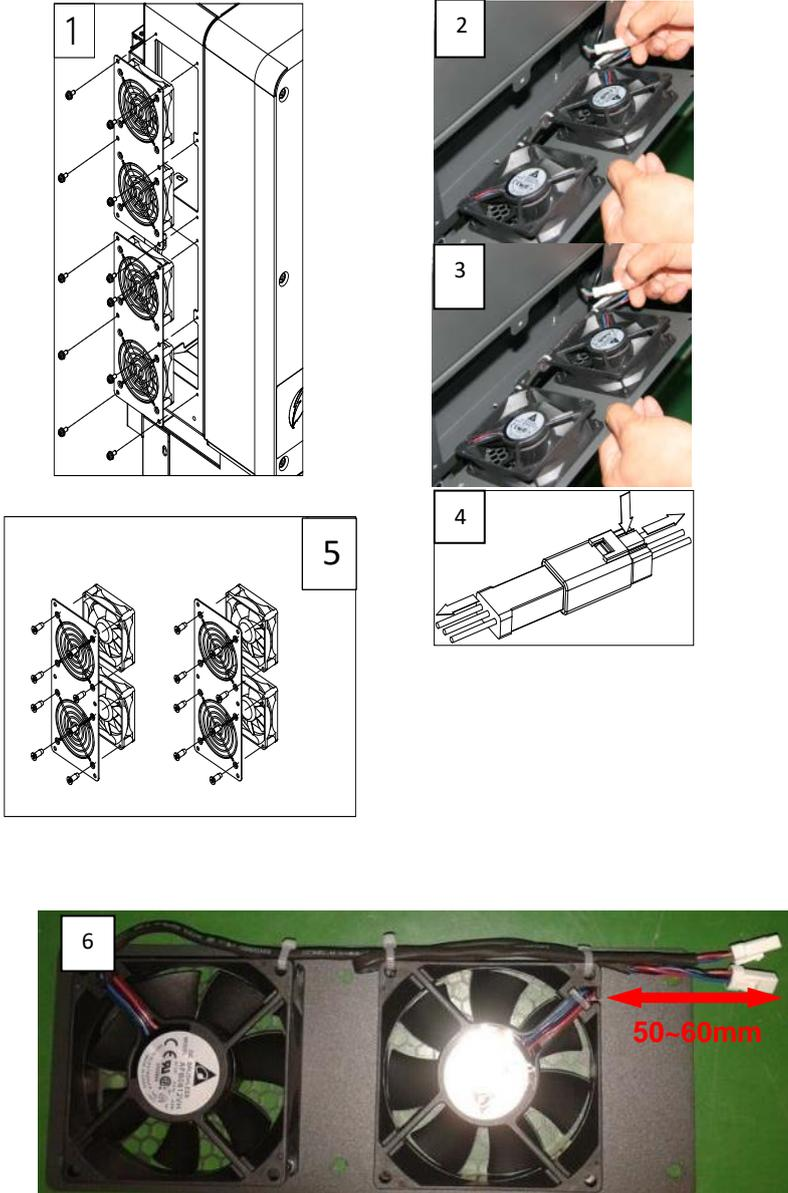
Figure 6.1 - Replace Cooling Fans
