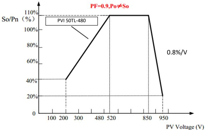
**Figure 7.1 - PVI 50TL kW and kVA Derating Curves of PV Input Voltage**
