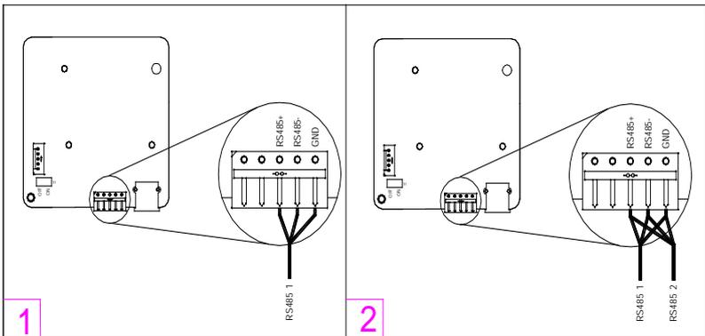
**Figure 2.41 - Communication Connections**
