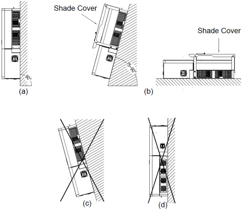
Figure 2.2 - Inverter Mounting
