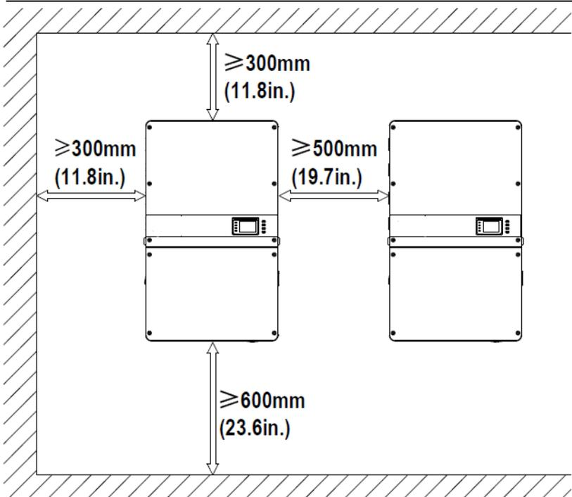
**Figure 2.3 - Inverter Wall Mounting Specifications**
