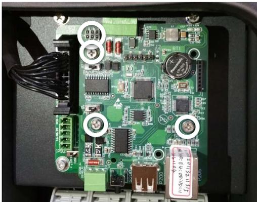
**Figure 2.48 - Ethernet Network Card Installed**
