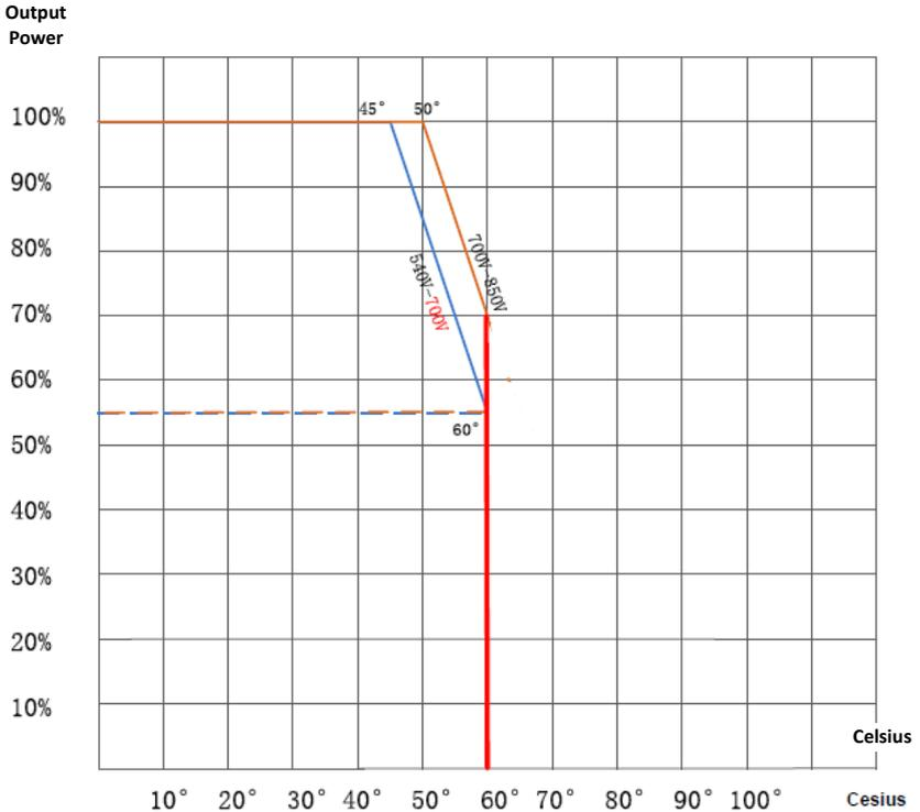
**Figure 7.3 - PVI 50/60TL Derating Curve with High Temperature**
