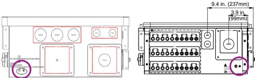
**Figure 2.38 - External Chassis Ground**
