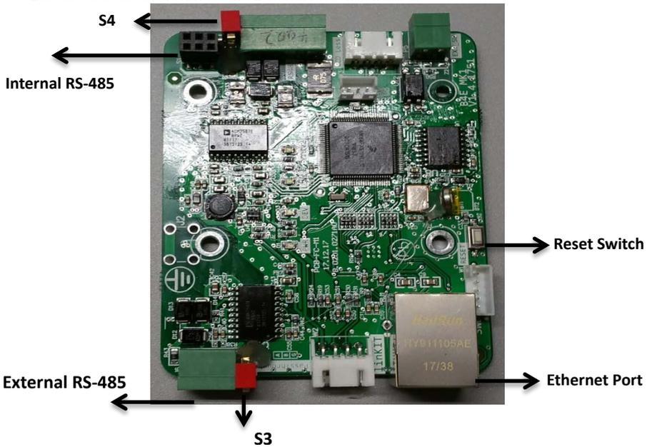
Figure 2.42 - Ethernet Network Card
