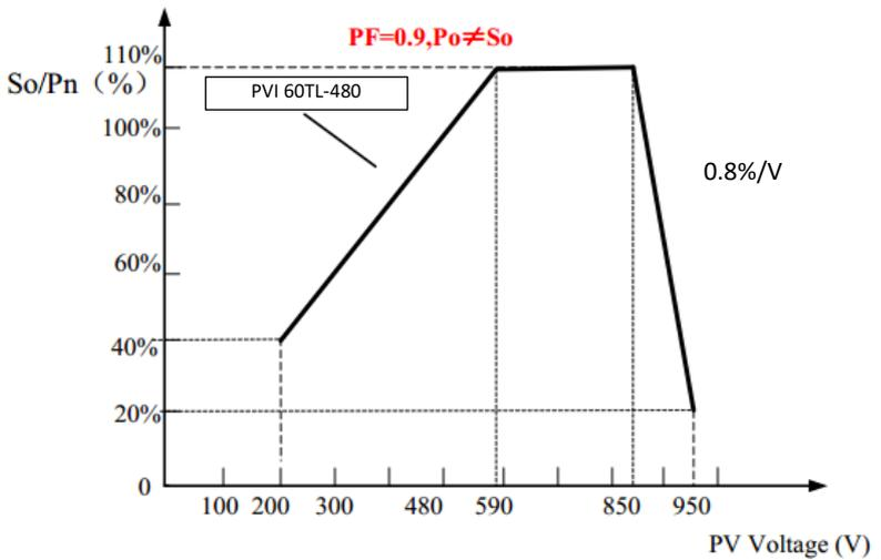
Figure 7.2 - PVI 60TL kW and kVA Derating Curves of PV Input Voltage
