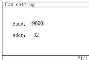
**Figure 3.2 – Selecting Baud Rate and Modbus ID**
