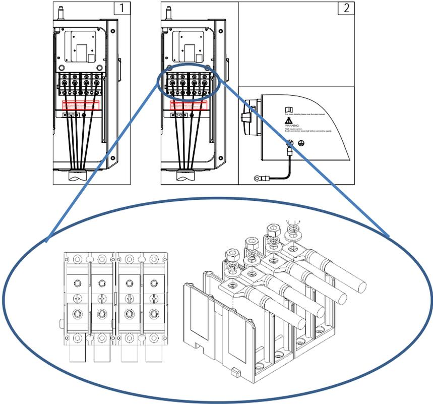
**Figure 2.36 - AC Output and Ground Cable Connections**
