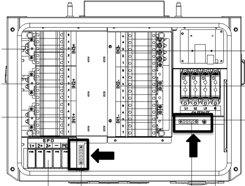
Figure 2.24 - Equipment Grounding Locations (Standard Wiring Box)
