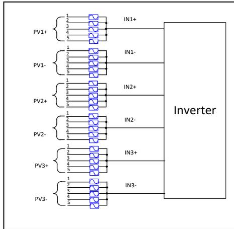
Figure 2.33 - Three MPPTs Operating Independently
