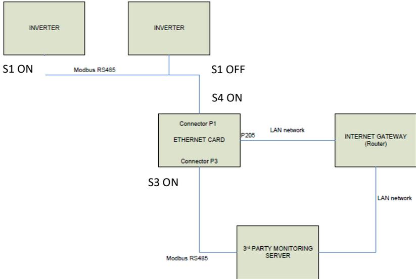
**Figure 2.44 - PVI 50/60TL Inverters in a RS-485 Daisy Chain Connection to an External DAS, Connectors and Termination Resistance Details**
