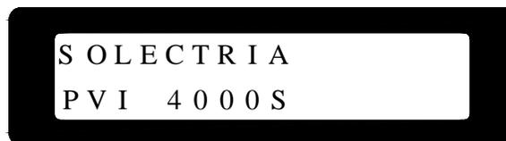
After 3 seconds, software versions of two embedded CPU's, Sequential and Current controllers, will be displayed on the LCD. Afterward, the serial number (S/N), the baud rate (BR) / address (ID) for the communication port will be displayed.
