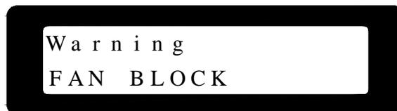
The messages for the **fault mode** are as follows. It shows the fault mode, serial number of the inverter, software versions of the sequential and current controllers and then the error messages which are listed in the Error Message Table 7.1.1.
