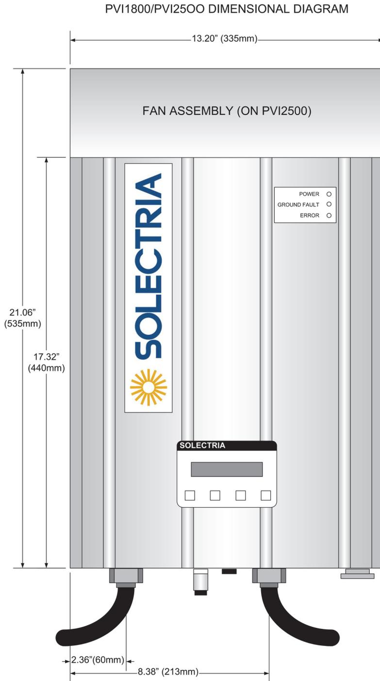
**Fig. 4 PVI 1800/PVI 2500 Dimensional Diagram**
