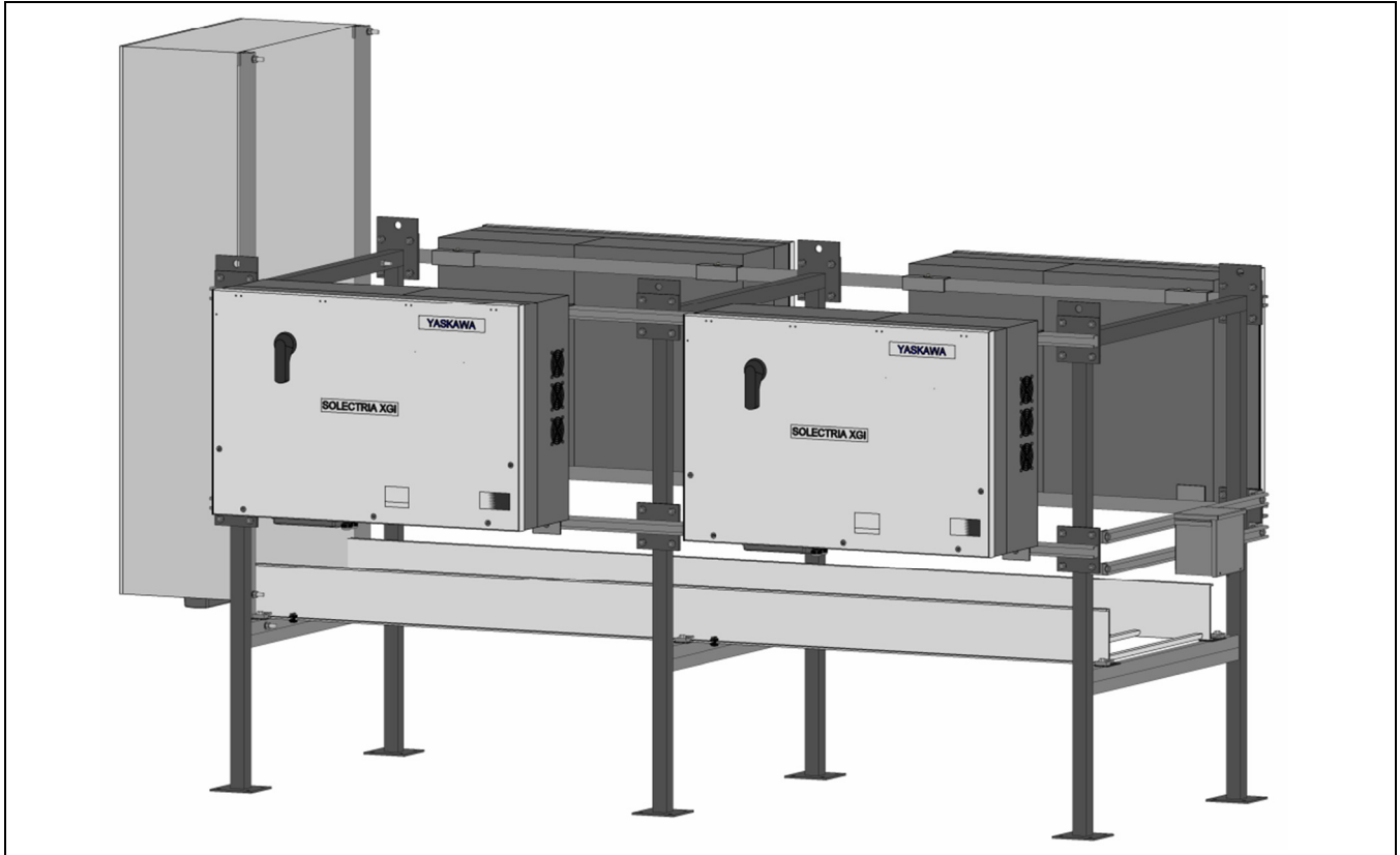
3-Inverter and 4-Inverter POWERACK: Isometric View
